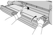
**12** While pressing down on the roll holder, pull the roll release lever forward to lock the paper guide.
